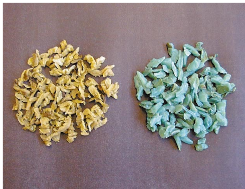
A copper adsorbent derived from sugar beet pulp produced at the BioComposites Centre, Bangor, UK
